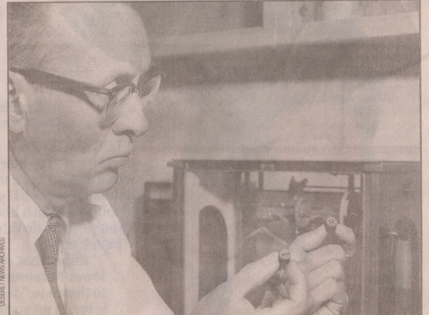
H. Tracy Hall holds 20-carat diamond cylinder, the world's largest known man-made diamond. The industrial stone was produced at a Provo lab in 1970.
